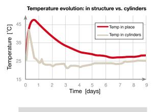
Given a concrete mix, temperature and strength development in structure vs. in-sample cylinders can vary consistently.
